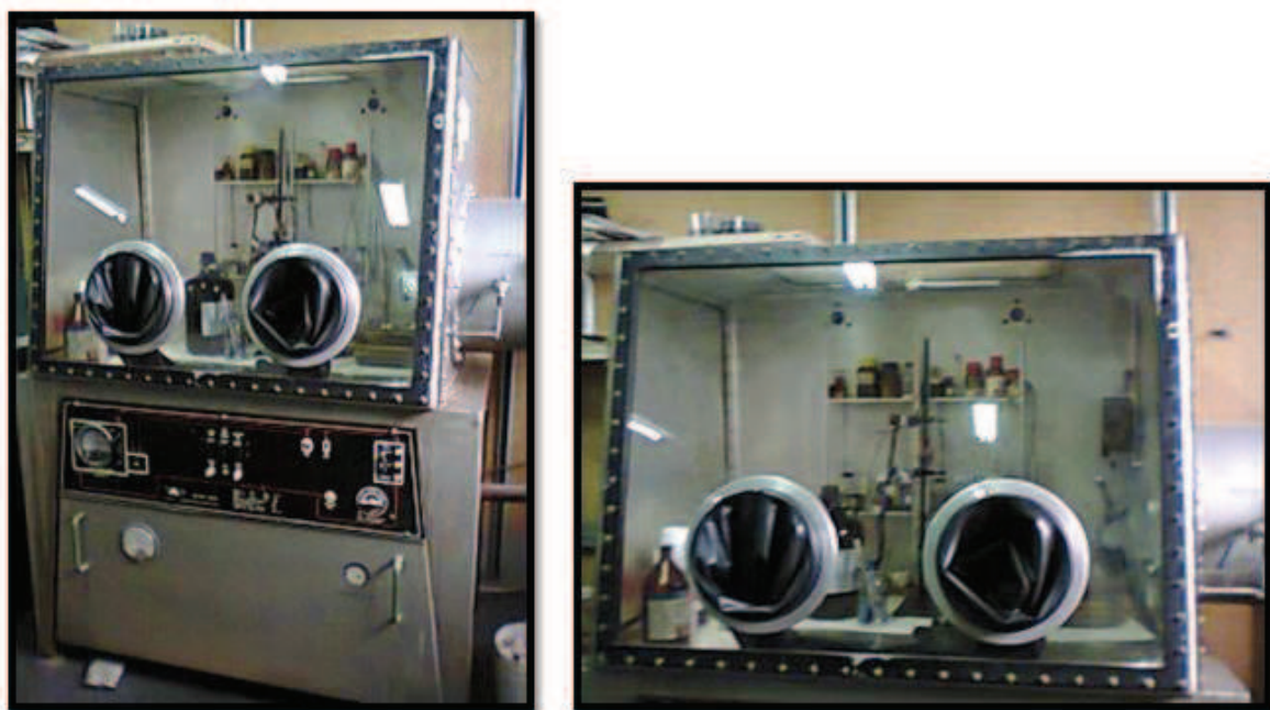
Figura 4.2. Caja seca. DRI-Train HE-193-1 Vacuum /Atmosphere Corporation
