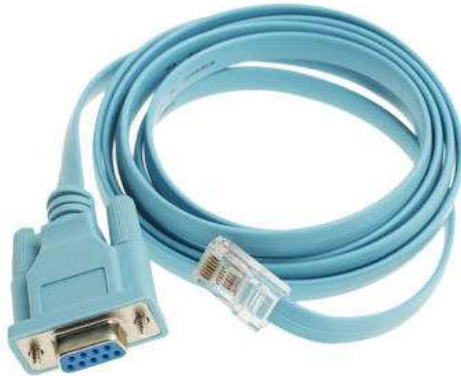
Figura 8.2: cable DB9 a RJ45
