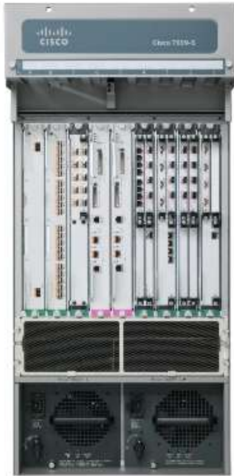
Figura 5.12: Cisco 7609-S Router
