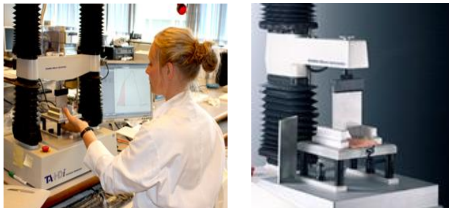
Figura 6: Set de Cuchillas Warner - Bratzler - Texturómetro Stable Micro Systems Texture Analyser, Model TA - XT plus.
